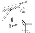
Release the trolley from the runner using the manual release pulley and move the door to the open position.
